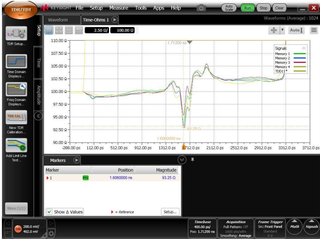
Figure 10. Typical differential TDR of TMDS, HDMI2.1-TPA-P mated to HDMI2.1-TPA-R at 70 ps Rise Time
