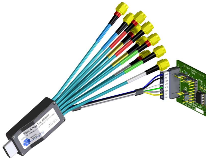
Figure 4. HDMIA2-TPA-E (E-EDID/Low Frequency Control Board) mated to a HDMIA2-TPA-12P (Plug) Test Adapter. NOTE: Coaxial cables shown are not to scale.
