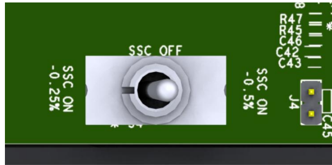
Figure 4. Receptacle REFCLK SSC Selection Switch (S4)
