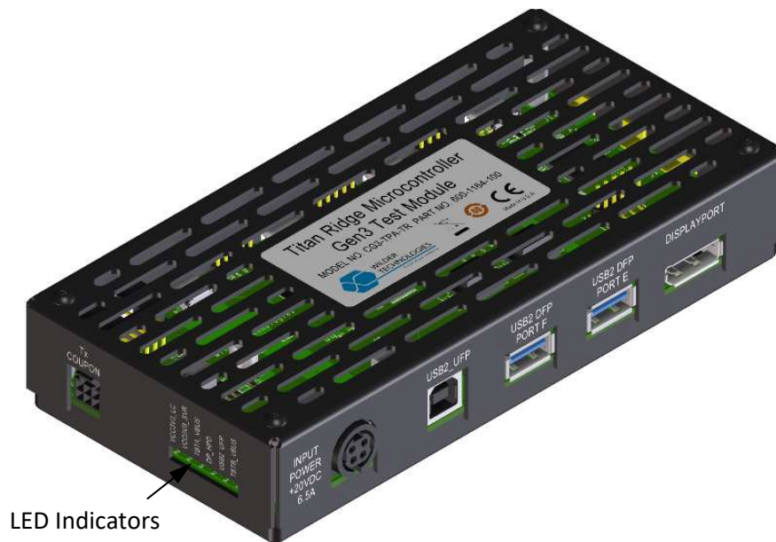
Figure 8. Titan Ridge Generation 3 Microcontroller LED Status Indicators
