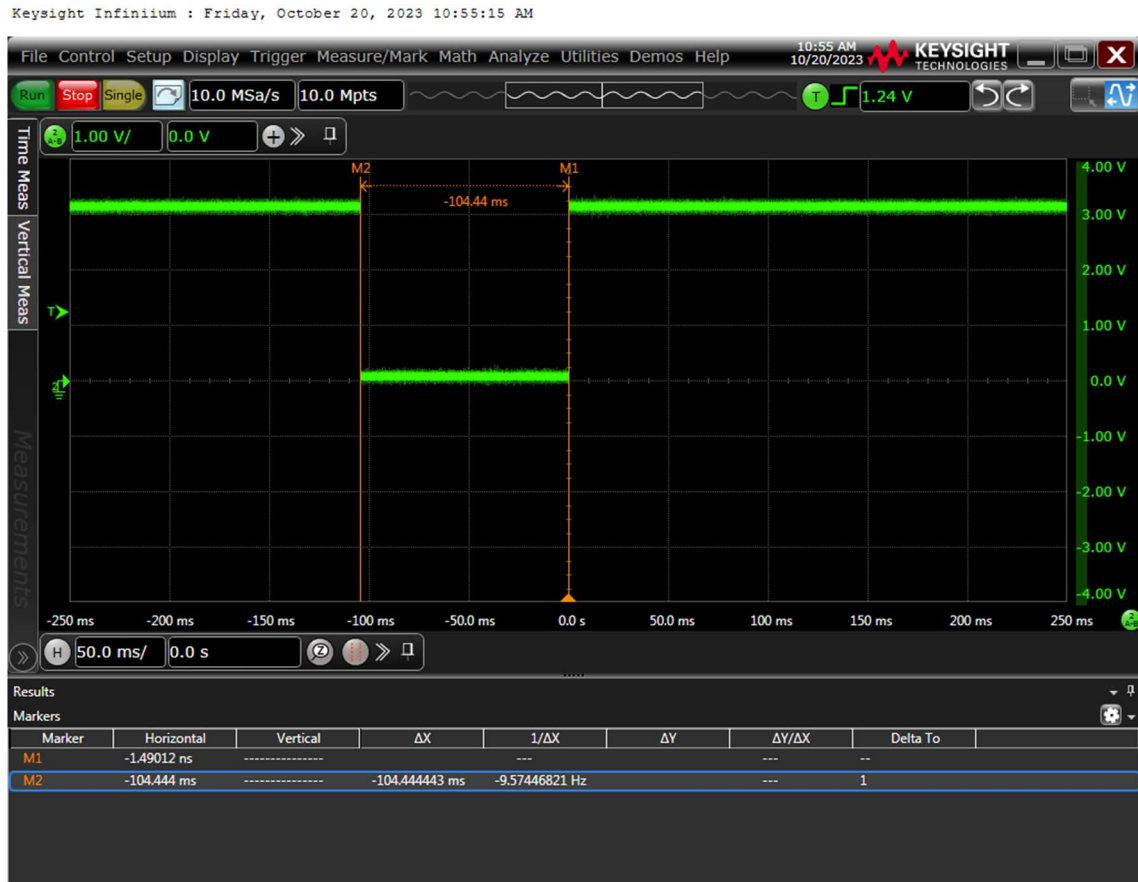
Figure 32: Delay Measurement After PERSTB Button Press on Real-Time Oscilloscope
