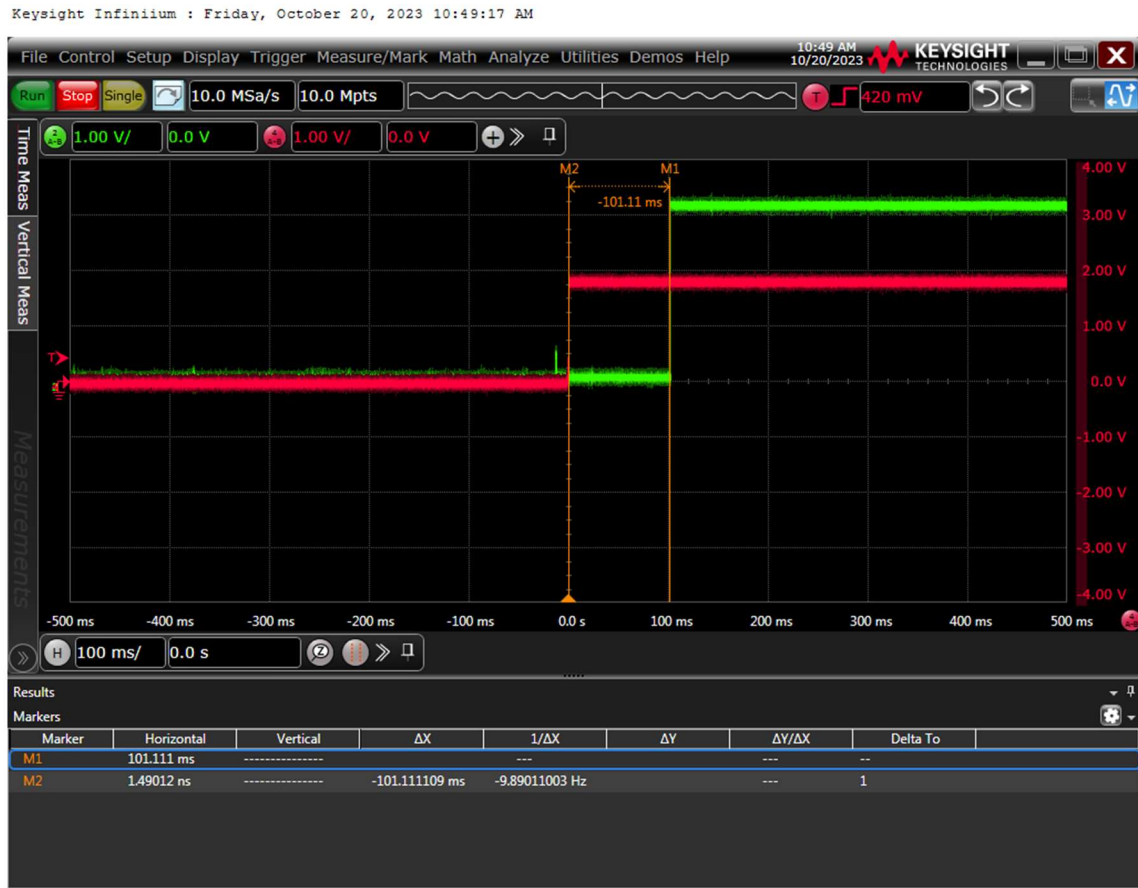
Figure 29: Delay Measurement between 1.8V rail start-up and PERSTnA Rise on Real-Time Oscilloscope
