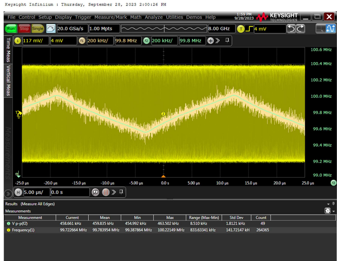
Figure 23: REFCLKB with SSC set at -0.5% down spreading
