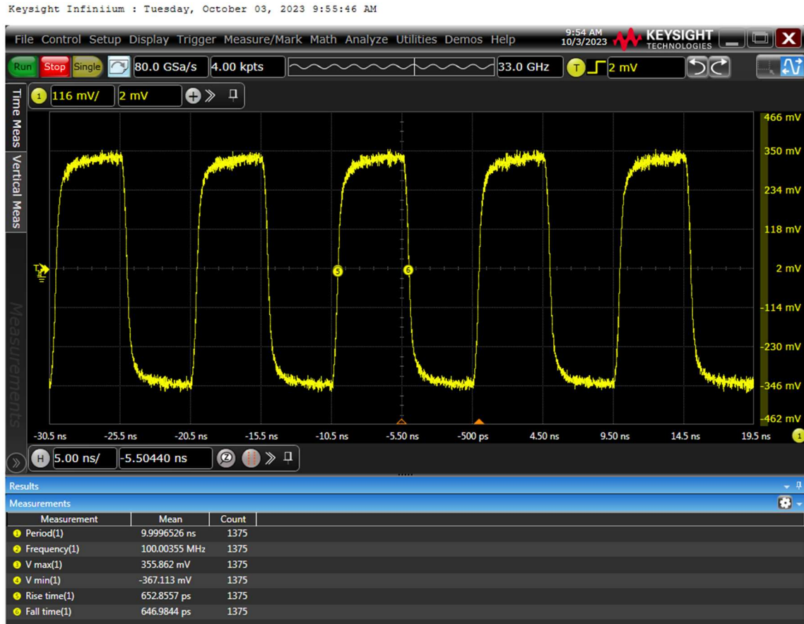
Figure 21: REFCLKB Characteristics on Real Time Oscilloscope
