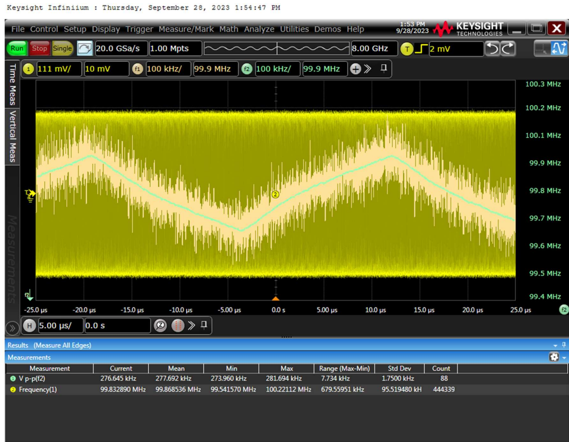
Figure 24: REFCLKA with SSC set at -0.25% down spreading
