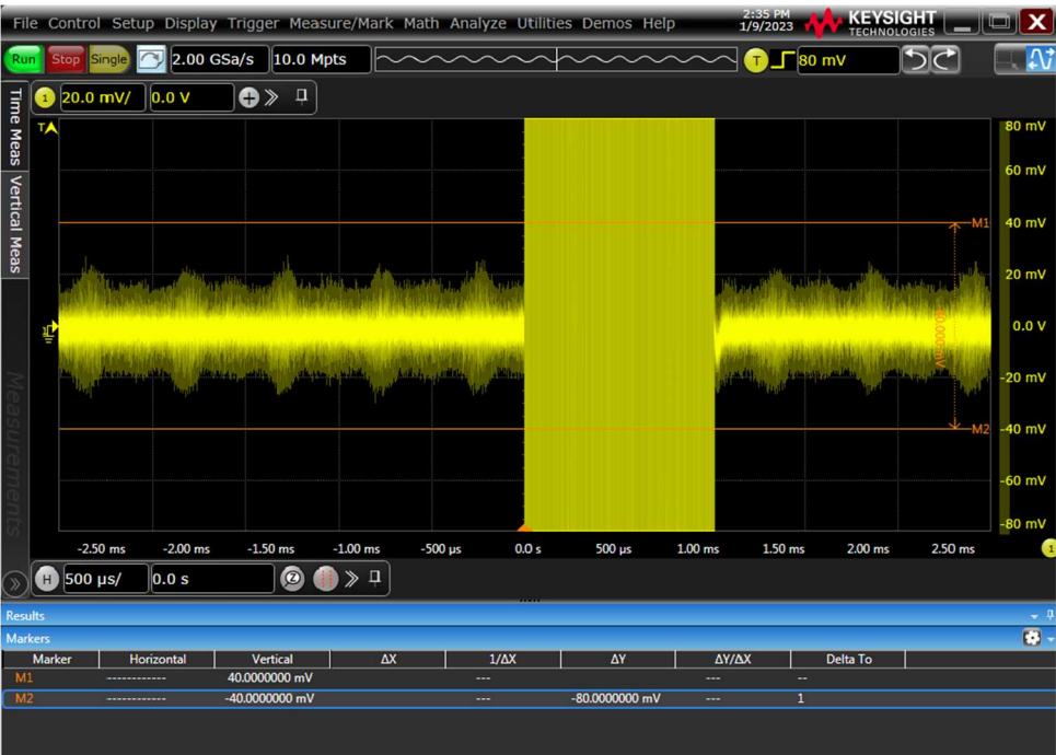
Figure 26: 40mV Noise Test of CMTS
