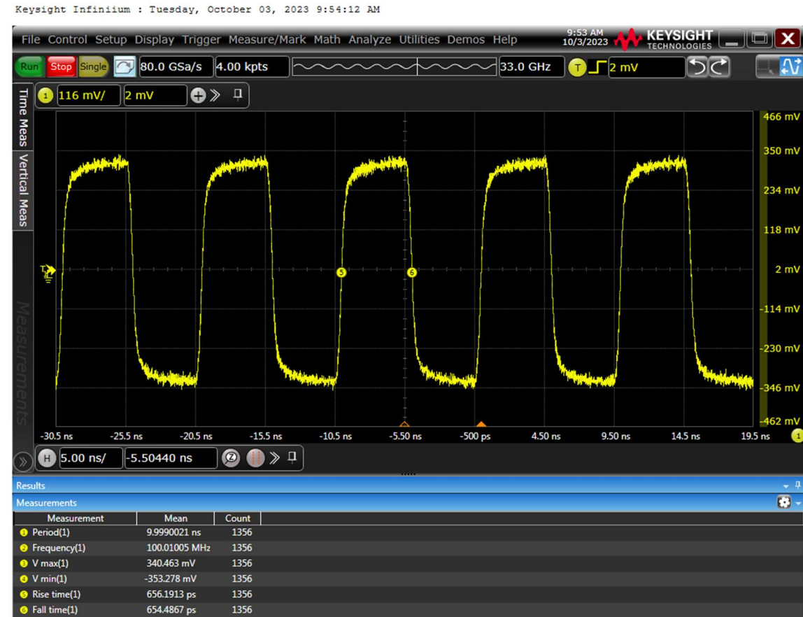
Figure 20: REFCLKA Characteristics on Real Time Oscilloscope
