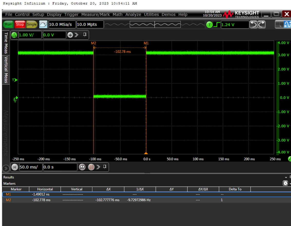
Figure 31: Delay Measurement After PERSTA Button Press on Real-Time Oscilloscope
