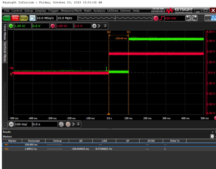
Figure 14. Automatic PERST Signal Delay (100 ms)
