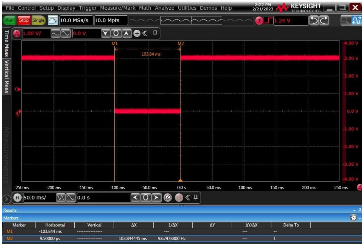
Figure 28: Delay Measurement After PERST Button Press on Real-Time Oscilloscope
