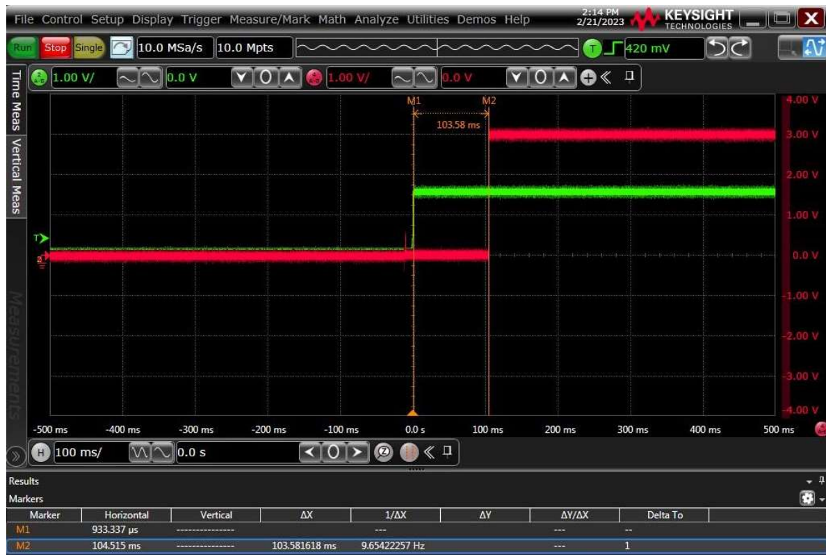
Figure 27: Delay Measurement between 1.8V rail start-up and PERSTn Rise on Real-Time Oscilloscope
