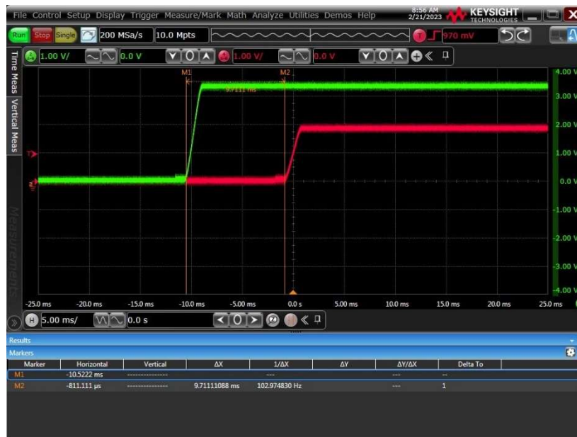
Figure 17: Voltage Rail Sequence Test Measurement
