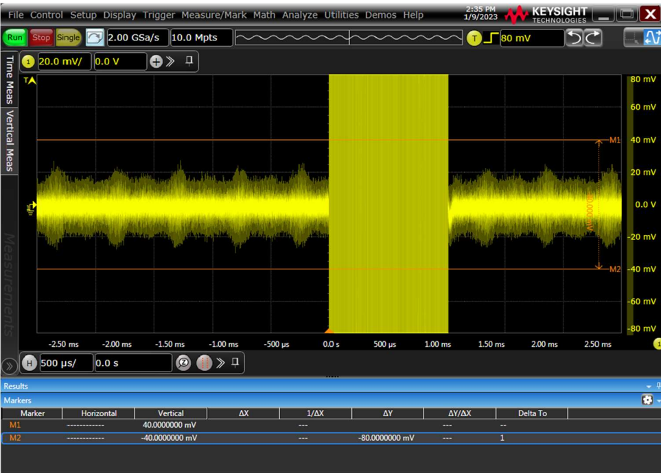
Figure 22: 40mV Noise Test of CMTS
