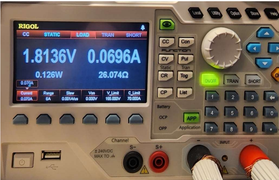
Figure 16: Electronic Load Results for the 1.8V Rail
