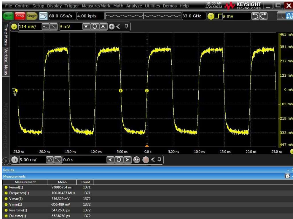
Figure 19: REFCLK Characteristics on Real Time Oscilloscope
