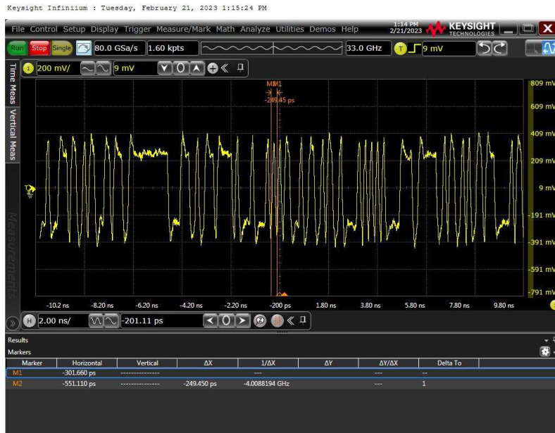
Figure 26: Measured Compliance Patterns on GEN3 AIC DUT (8.0GT/s PCIe 3.0 Preset 0)
