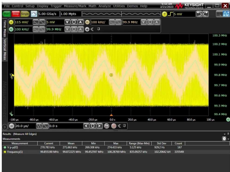
Figure 21: REFCLK with SSC set at -0.5% down spreading
