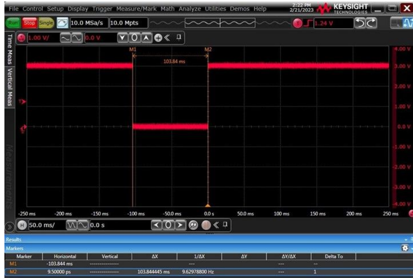
Figure 17. Manual PERST Signal (100 ms)
