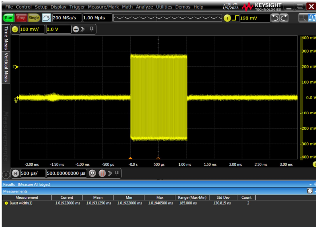
Figure 5. CMTS Pulse Duration (1 ms)
