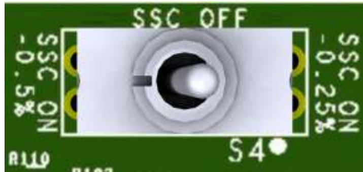
Figure 13. CBB REFCLK SSC Selection Switch (S4)
