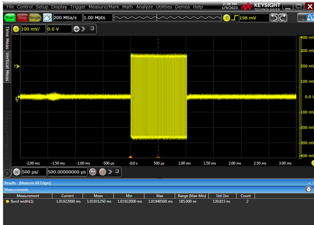
Figure 5. CMTS Pulse Duration (1 ms)
