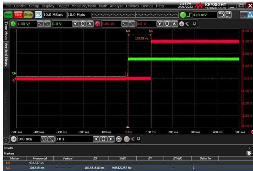
Figure 16. Automatic PERST Signal Delay (100 ms)
