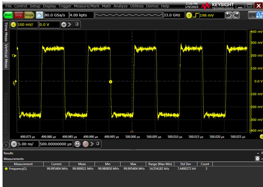
Figure 6. CMTS Frequency (100 MHz)
