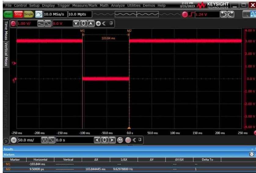
Figure 17. Manual PERST Signal (100 ms)
