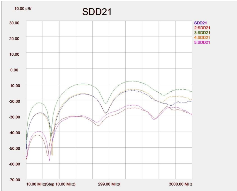
Figure 13. Typical Differential NEXT for section 4, with mated connectors, adjacent differential pairs, both transmit and receive terminated at both ends. (Measured with two ETH-TPA-RJ45 calibrated to the pads of the plugs.)
