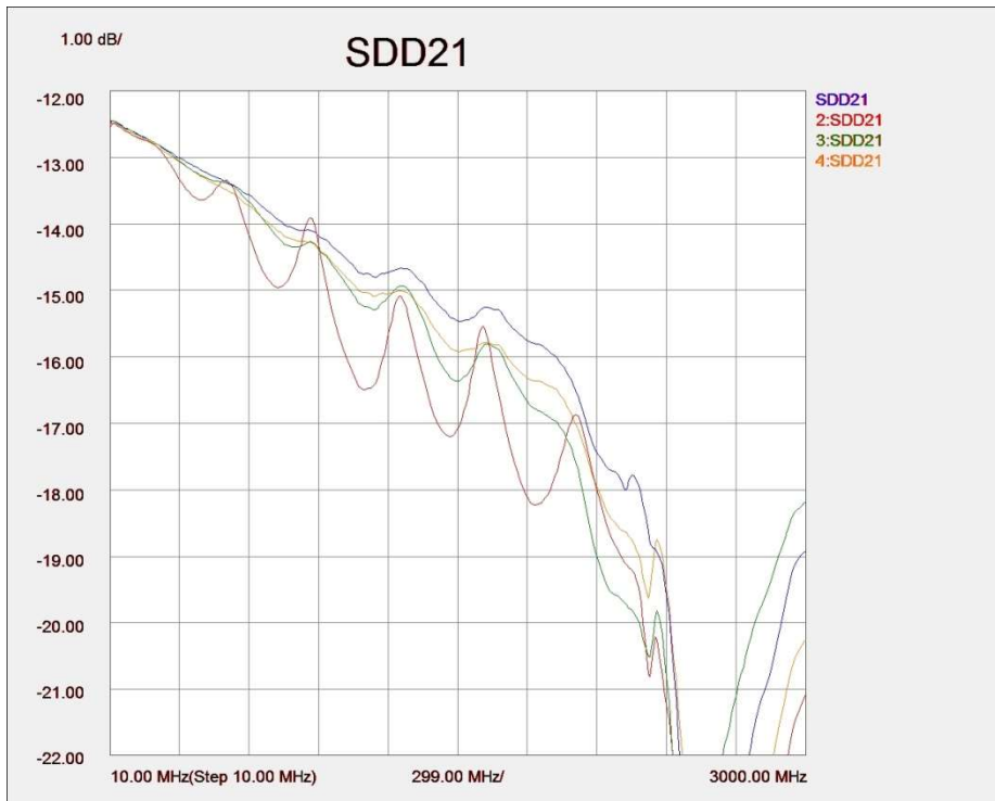
Figure 8. Typical section 2 balanced insertion loss of coupler FWD output. (Measured with one ETH-TPA-RJ45.)
