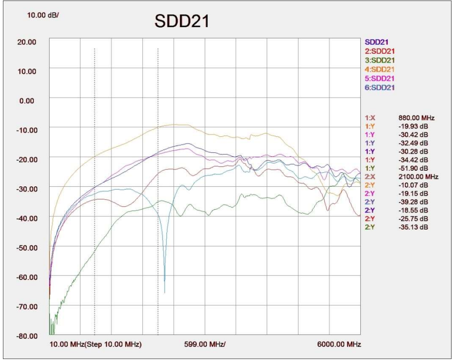
Figure 10. Typical Differential NEXT, for RJ-45 TPA, with mated connectors, adjacent differential pairs, both transmit and receive terminated at both ends (using Agilent 10GBase-T Ethernet Test Fixture p/n U7237-66501).
