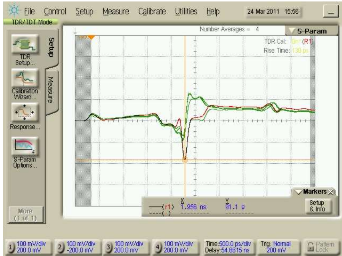
Figure 13. Typical Differential TDR of TPA-P connected to TPA-R at 130 ps Rise Time
