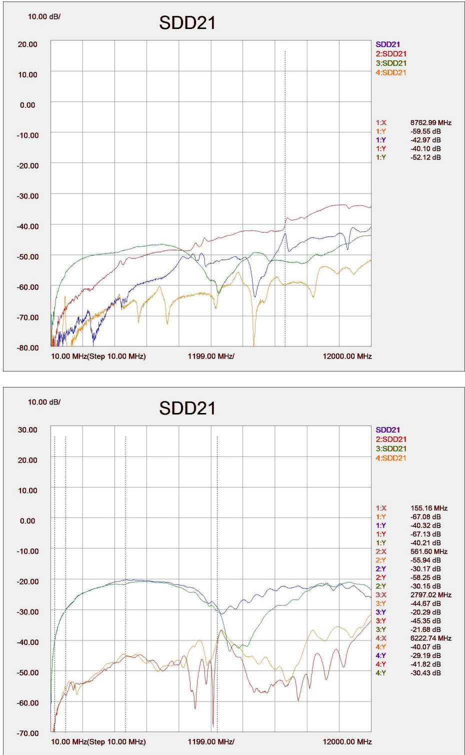
Figure 21. Typical Differential NEXT of HEAC to D2, without connector (top) and with mated connectors (bottom); all lanes terminated at both ends
